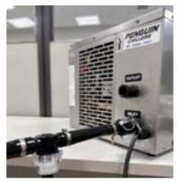
After you secure the camlock fitting in place, remove the metal pin (not in the video) and put it through the hole on the camlock fittings itself to ensure you have a good hold.
